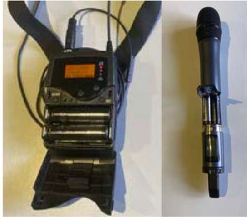
Picture 8: To change the batteries: Flip the collar microphone open; unscrew the handheld mic at the bottom
