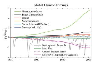
But since the Industrial Revolution, sulfate aerosols have caused other changes in the atmospheric composition. Power plants burning high-sulfur coal produce SO<sub>2</sub>, which mixes with cloud droplets to produce reflective sulfate droplets and acid rain. Moreover, aerosols have an indirect effect: smaller cloud droplets create brighter clouds and they require more collisions to crete droplets large enough to precipitate. Consequently clouds last longer.
