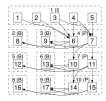
Fig. 3. Dependency graph  $G_1$  obtained by encoding 10 frames of the Foreman video sequence with H.264. The vertex labels show the packet numbers in stream order, the dashed boxes indicate the frames with the frame number relative to the first encoded frame and the frame type in parentheses. For clarity, no redundant edges are shown.
