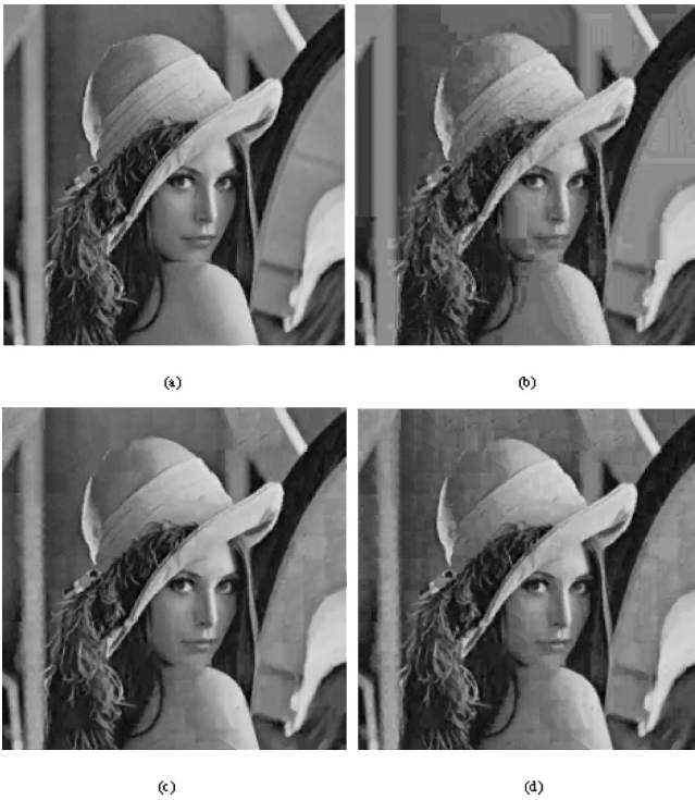
Fig. 3 (a) The collage image of FIC A, PSNR=33.38 dB; (b) the decoded image of FIC A, PSNR=28.92 dB; (c) the collage image of FIC B, PSNR=32.15 dB; and (d) the decoded image of FIC B, PSNR=31.51 dB.
