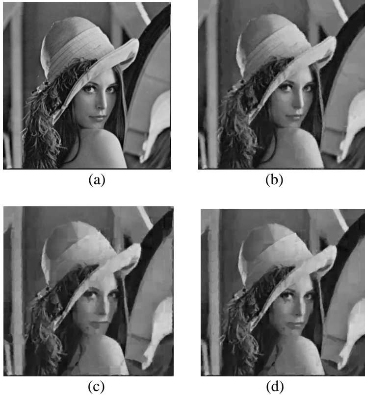
Fig. 6. (a) The original image (b) Reconstructed by the method presented in the paper (c) Reconstructed by the spatial domain fractals (d) Reconstructed by DCT domain fractals.
