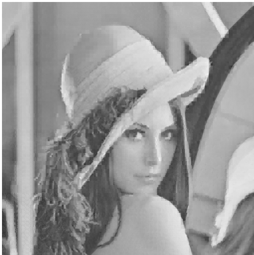
Fig.2c. Vector distortion fractal coding using fixed partition : range block 8×8, domain block 16×16, \Delta h, \Delta v = 16 , compression ratio = 46.54, PSNR = 26.90 dB.
