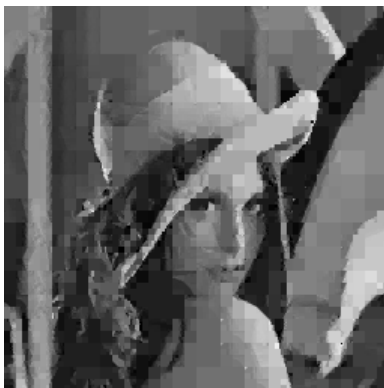
Figure 3: The 256x256 “Lena” Image Compressed with Wavelet Aided Fractal Compression. The Haar wavelet was used. Compression ratio: 43:1, RMS error: 14.8.
