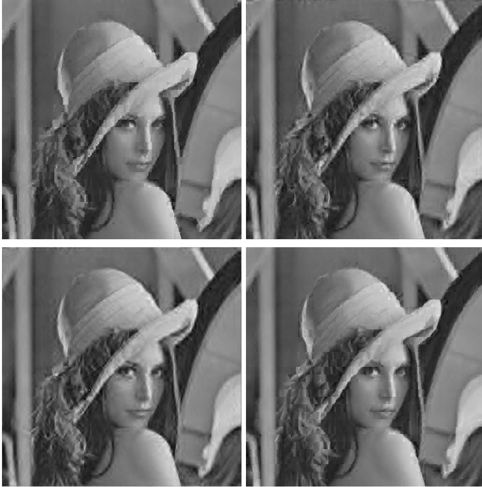
Figure 10. Top: Generalized IFSW approximations with (k_1^*, k_2^*) = (4, 5) . The three child blocks A_{k_2^*ij}^\lambda have independent scaling factors \alpha_{ij}^\lambda but a common parent block. Left: Haar basis, d_2 = 12.5 , PSNR= 26.2. Right: Coifman-6 basis, d_2 = 11.8 , PSNR= 26.7. Bottom: Left: (4, 5) IFSW approximation as above but with Daubechies-10 basis, d_2 = 11.4 , PSNR= 27.0. Right: Place-dependent IFSM (Bath Fractal Transform). 32 \times 32 pixel parent cells mapped to 16 \times 16 pixel child cells. Each child cell has three scaling factors. d_2 = 12.5 , PSNR= 26.2. The compression ratios (unoptimized) are roughly 45:1.
