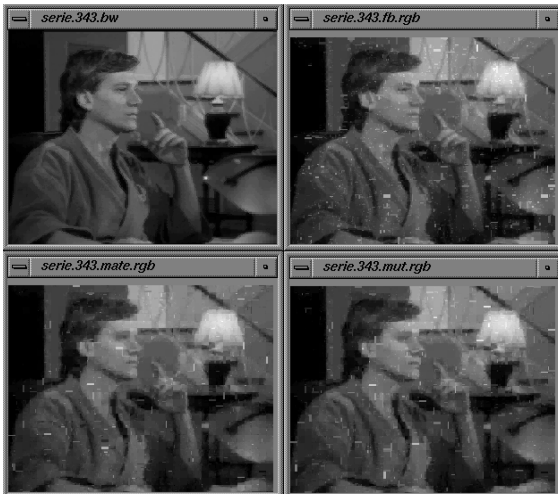
Figure 8: Original Image (above left) compared with the images obtained by using Barnsley's algorithm (above right) and GA's using modified mating operator (below left) and modified mating and mutation operators (below right).
