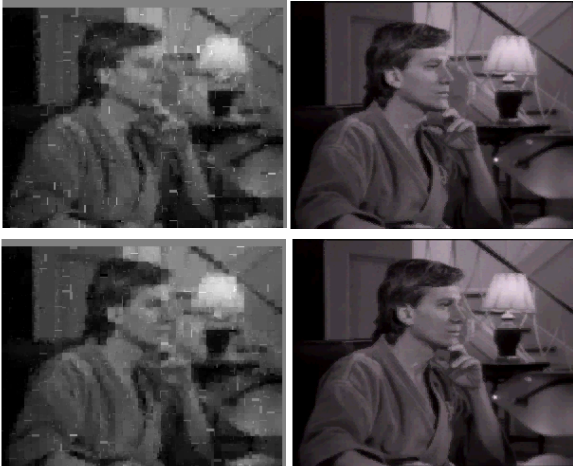
Figure 10: Image sequence: last two of four consecutive video frames, in compressed and original form. The second mutation operator and stored initial populations were used.
