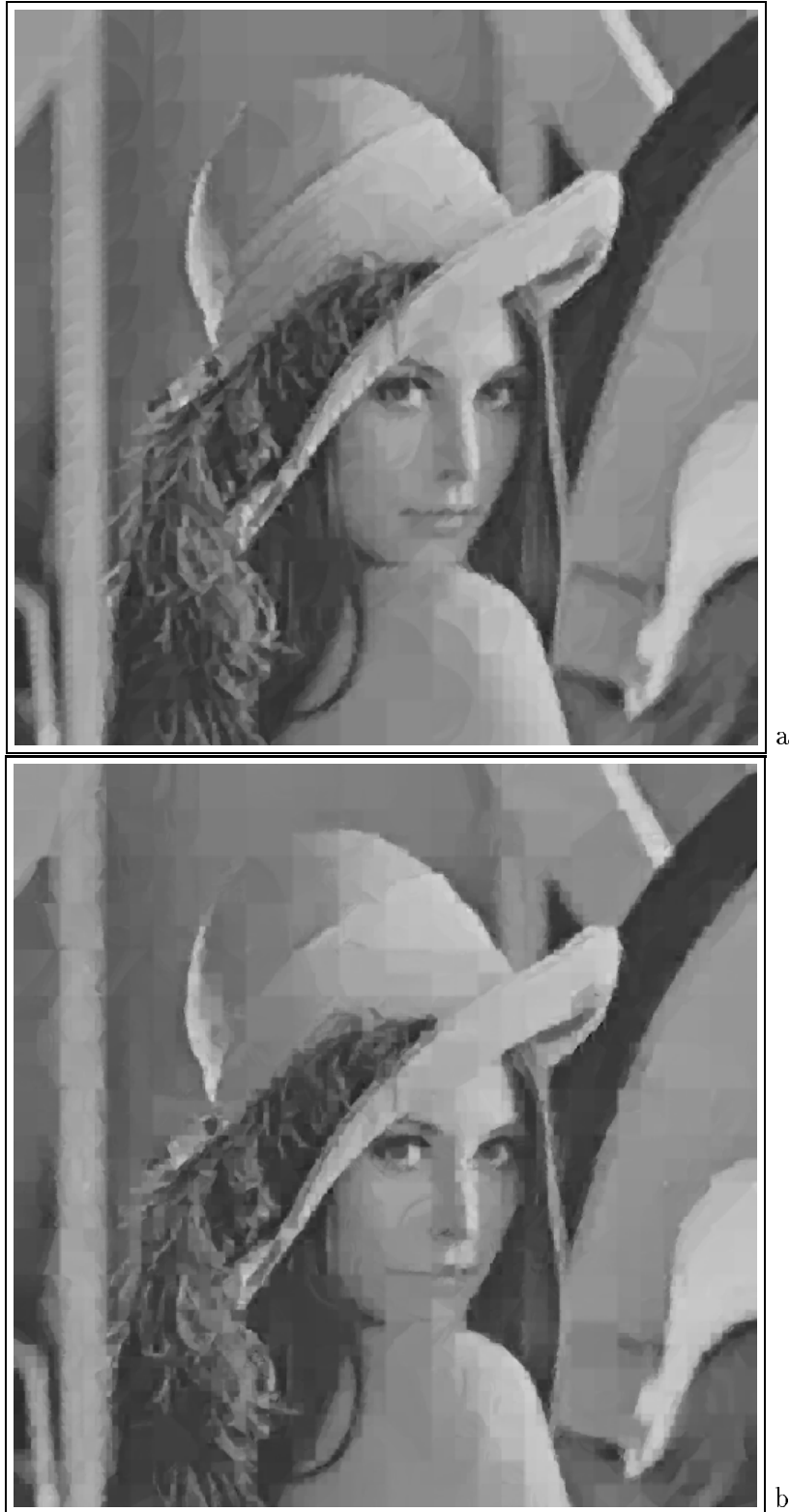
Fig. 5 Lena 512 \times 512 coded with a compression factor of 50.9 and PSNR = 28.76dB with the new algorithm (a), and at PSNR = 27.9 dB with the classical quad-tree algorithm (b). The image (a) was generated with the use of only 32+32+32 = 96 domain vectors
