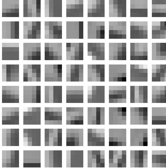
Figure 3: Visualization of a shape codebook in mean-removed shape-gain vector quantization. It consists of 64 blocks of size  $4 \times 4$  pixels with zero mean and unit variance. For the display the vector components have been multiplied with a gain of 180 and are added to the mean of 127.
