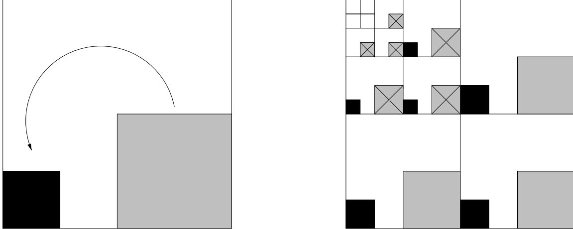
Figure 15: Left:  $4 \times 4$  range (black),  $8 \times 8$  domain (shaded). Right: the corresponding wavelet subtrees; the crossed shaded parts of the domain wavelet subtree can be used for a prediction of the range wavelet subtree.
