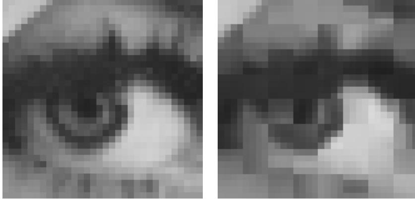
Figure 2: Standard vector quantization of a section of the Lenna test image (original on left) using a codebook of 512 blocks of size  $4 \times 4$ . The attainable PSNR with this approach is about 31.2 dB for the Lenna test image.
