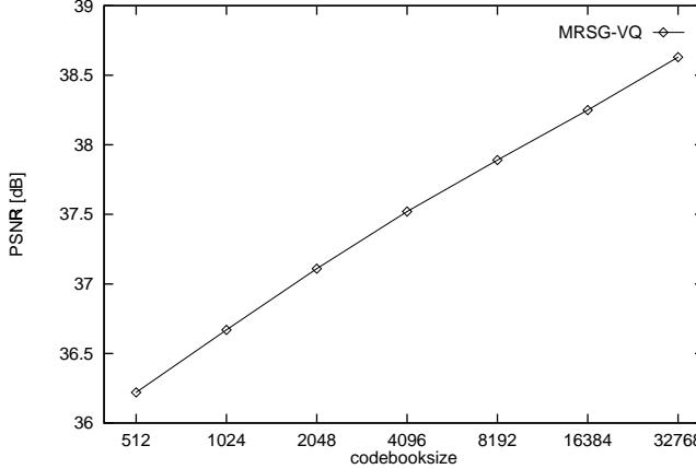
Figure 6: Codebook size vs. distortion curve for *MRSG-VQ* using blocks of size  $4 \times 4$  and shape codebooks of various sizes. The uniform scalar quantizers for the gain and the mean use 32 and 128 levels respectively. The test image is  $512 \times 512$  Lenna.
