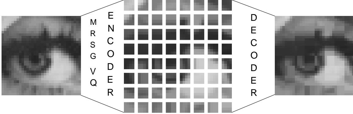
Figure 5: Visualization of the MRSG-VQ codec. The test image Lenna is encoded using the shape codebook of size 64 shown in Figure 3. The uniform scalar quantizers for the gain and the offset use 32 and 128 levels respectively. The picture shows only an enlarged section (32 by 32 pixels) of the entire image in order to better see the pixels and the image blocks. The PSNR for the entire image approximation is 34.6 dB
