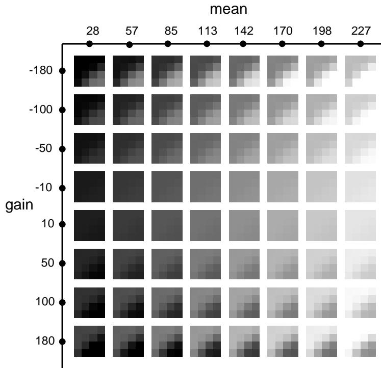
Figure 4: Visualization of the MRSQ-VQ product code blocks for the second shape block in the third row of Figure 3. The scalar codebooks for the gain and mean contain only eight values as shown in the graph.
