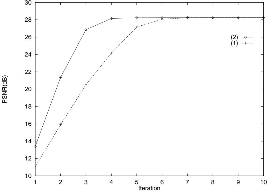
Figure 16: PSNR vs. iteration step for the  $512 \times 512$  Lenna image. The image was encoded with Fisher's quadtree code with the default parameters (three-level quadtree, one-class search). Curve (1) corresponds to the conventional decoding, curve (2) to the method with codebook update.
