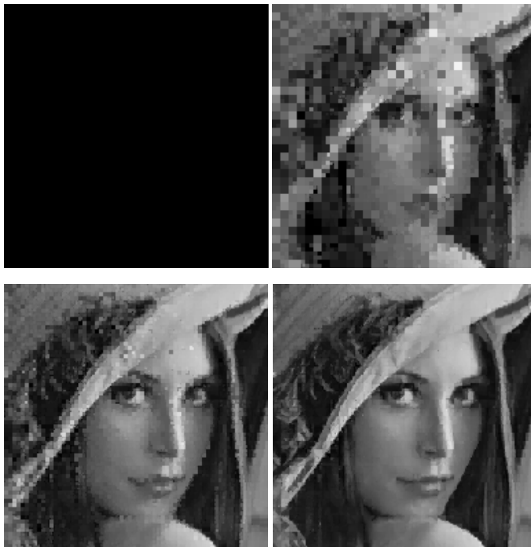
Fig. 3. Iterations 1,2,4 of a code for "Lena" applied on a gray image ( n=8 ).
