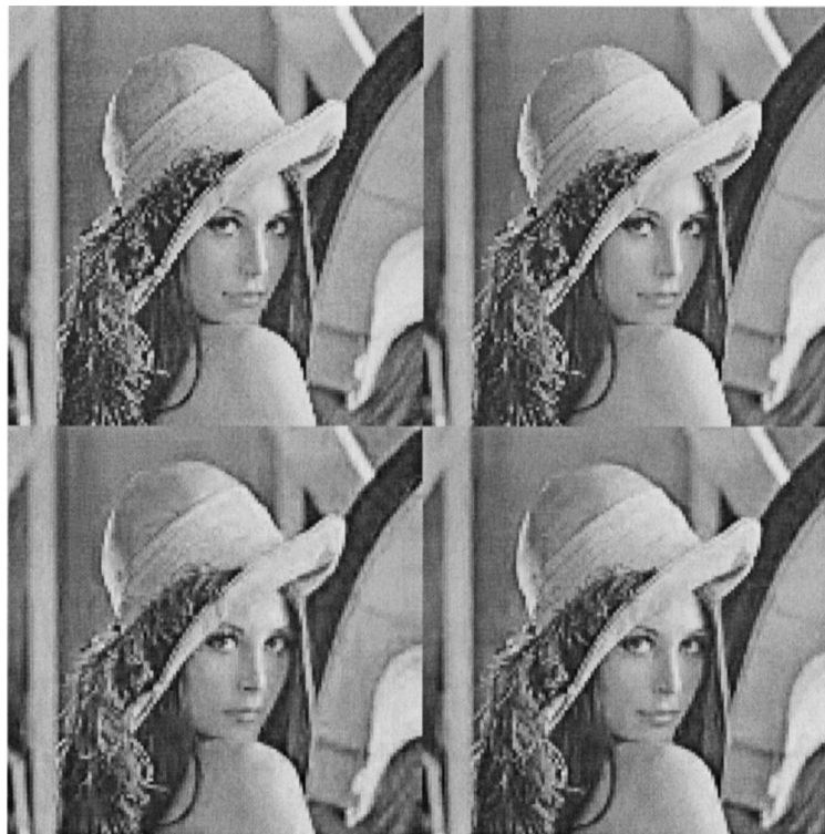
Fig. 3. 8-Bit image ‘Lena’ for several compression factors using 16 \times 16 blocks. Clockwise, from upper left: original, 0.65 bpp, 0.34 bpp and 0.21 bpp.
