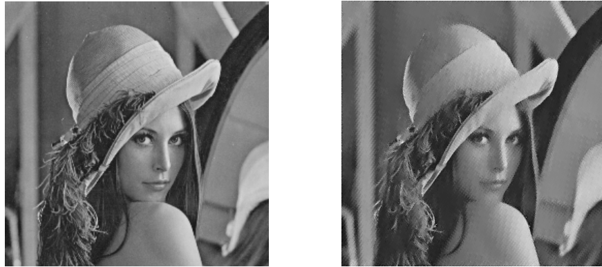
Fig. 6. Wavelet compression on dust. Left: Original 512 \times 512 of Lena. Right: Reconstruction of Lena from pruned wavelet tree. PSNR=27.22 dB.
