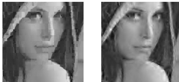
Fig. 5 - parts of the reconstructed image "lena" (a) Haar DWT, L=4 (b) Adelson 9 Taps, L=4
