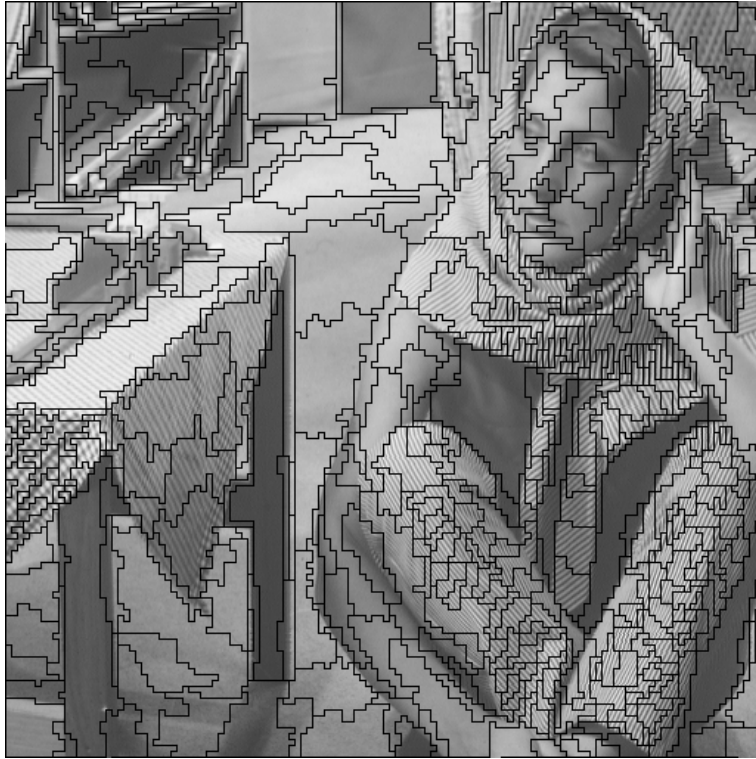
Figure 1: Partitioning of the 512 \times 512 Barbara image in 600 ranges of various sizes and shapes.
