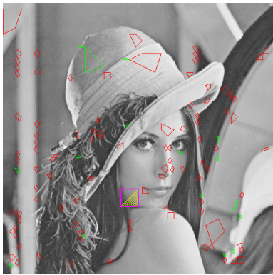
Figure 6: Associations at the end of the encoding step: the bold-lined square is mapped onto each fine quadrilateral, and the hatched triangle onto each fine triangle
