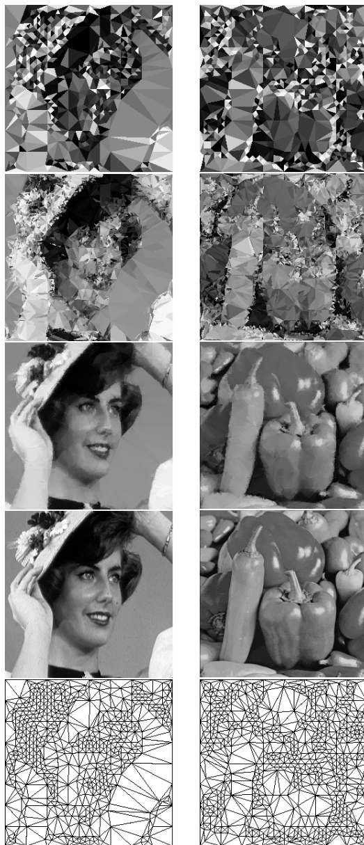
Figure 2: Decoding results. From top to down: first, second and tenth iteration starting with a white image, the original image, and the associated partition R . Left: Compression ratio = 18.3, PSNR = 27.4 dB. Right: Compression ratio = 15.6, PSNR = 27.3 dB
