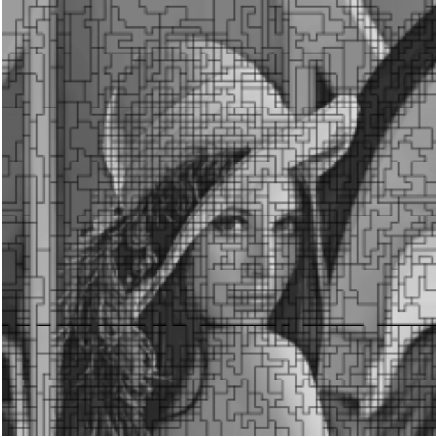
Figure 2. Partitioning with 2000 ranges (N=2, compression ratio 33.77, PSNR=30.96 dB)
