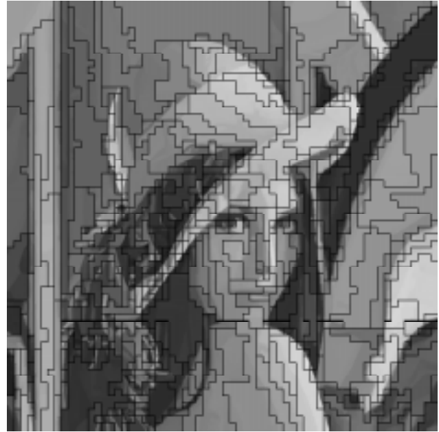
Figure 8. Decoded 512×512 Lena image with 500 ranges (compr. ratio 97.16), \alpha=0.10 , N=2, PSNR=27.24 dB, total encoding time 510 sec.
