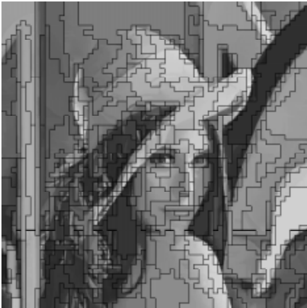
Figure 3. Partitioning with 500 ranges (N=2, compression ratio 97.16, PSNR=27.12 dB)
