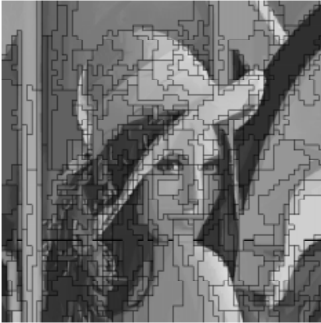
Figure 7. Decoded 512×512 Lena image with 500 ranges (compr. ratio 97.16), \alpha=0.25 , N=2, PSNR=27.21 dB, total encoding time 1107 sec.
